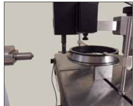
CNC controlled external taper ring measurement
