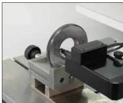
Checking of taper thread ring gauges (TA-MS-381/TEL75)
