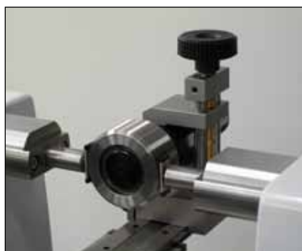
Calibration of thread plug gauges (3P/0.17-3.2/S6.5/TA-SU-315)
